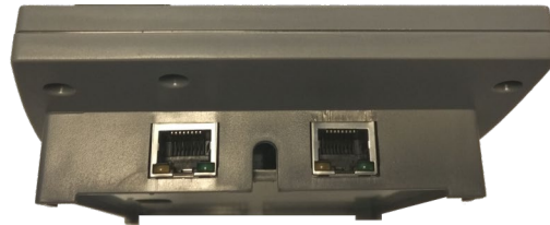
L-Net ports on the back side of 4E-FM
